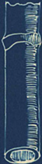
TUBE DRILL USED WITH SAND AND WATER
