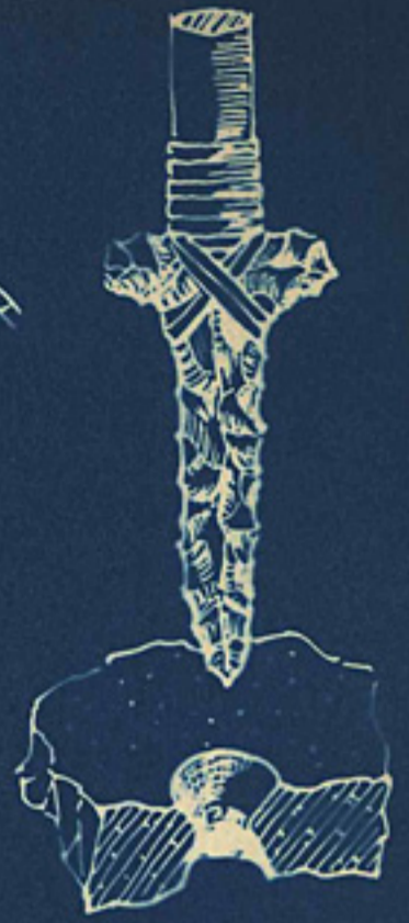
STONE DRILL FIXED ON SHAFT AND HOLE IN STONE MADE WITH THIS DRILL
