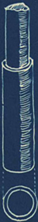
TUBE DRILL USED WITH SAND AND WATER
